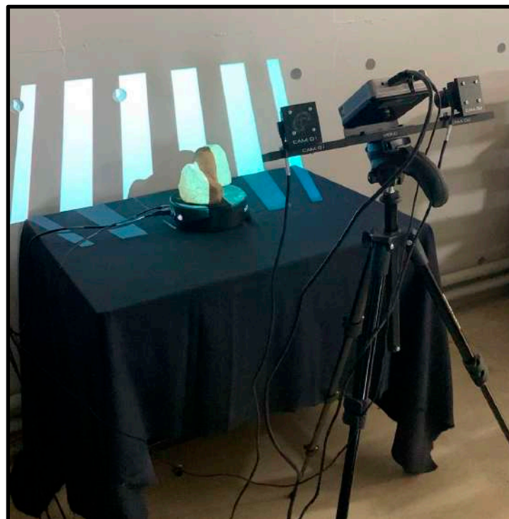
Figure 2. Scanning a fossilized coral colony with Scan-in-a-box structured light scanner.
